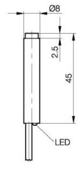
Inductive Sensors BES 516-396-EO-C-PU-03 D8 x 45 normally-open Sn=2,5mm unshielded
